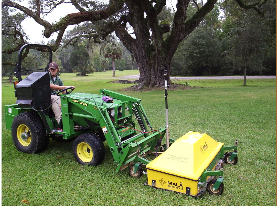
The GEL Geophysics crew using the CART system to scan the ground.
